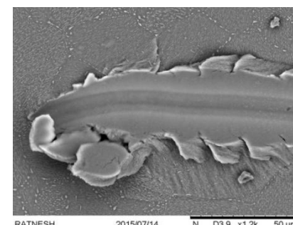
Scanning Electron Microscope(SEM) image of Nanoscratch
